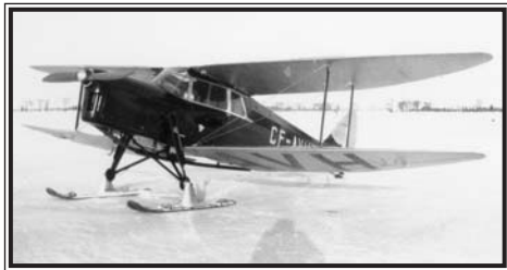
The first Canadian D.H. 87A Hornet Moth, CF-AVH, on skis with the original tapered wings, circa 1935. Jack McNulty Photo
