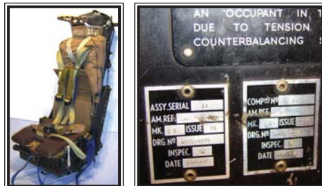
Avro Arrow ejection seat and 1958 data plates
