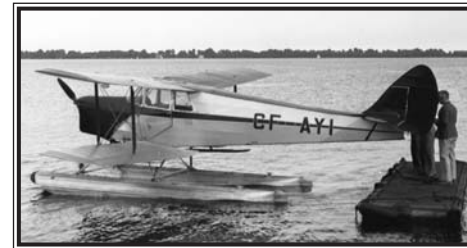
CF-AYI was the first Hornet Moth fitted with floats by Fairchild. It is pictured in Toronto Harbour on July 18, 1937. Jack McNulty Photo
